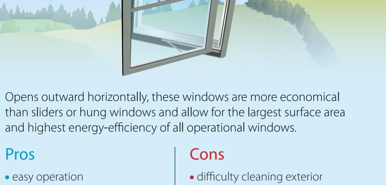
good ventilation • hardware wear and tear • must be closed in high wind • interior screens excellent security protrudes outward
